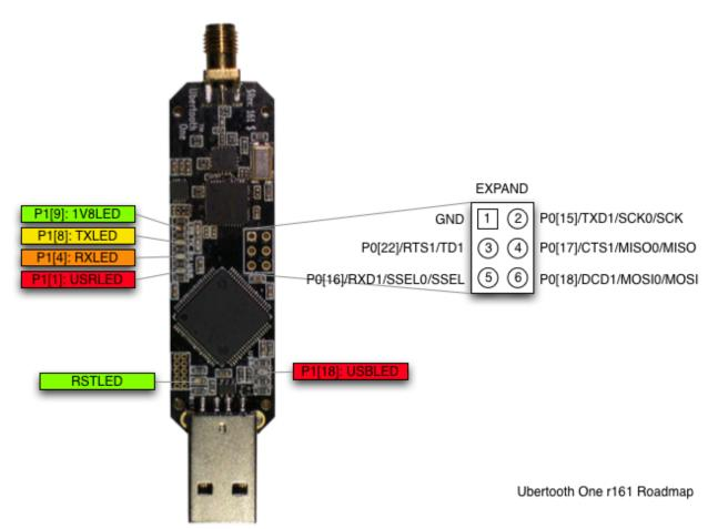
This diagram shows the location of LEDs and the pins of the expansion connector. LED guide:
