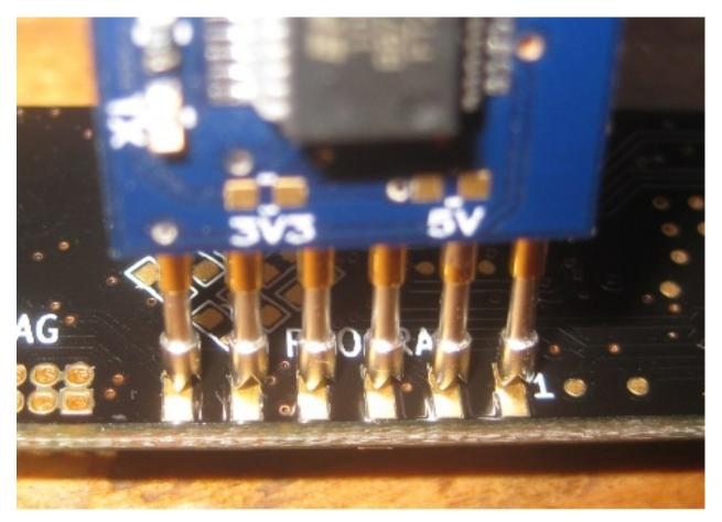
Warning: Code loaded via ISP will blow away the bootloader. It is generally recommended to use this method only for installing the bootloader itself.
